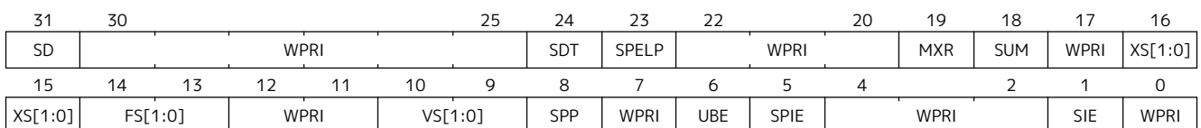
Figure 42. Supervisor-mode status ( sstatus ) register when SXLEN=32.
