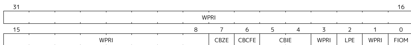
Figure 55. Supervisor environment configuration register ( senvcfg ) for RV32.
