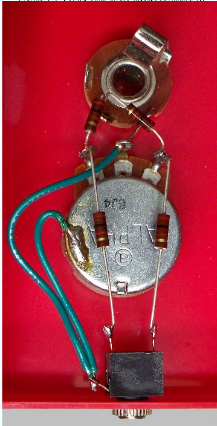
Figure 7-4. Sound card audio interface wiring (II)
