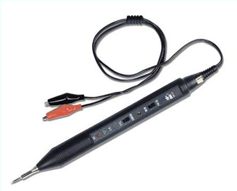
Figure 2-4. A typical logic probe
