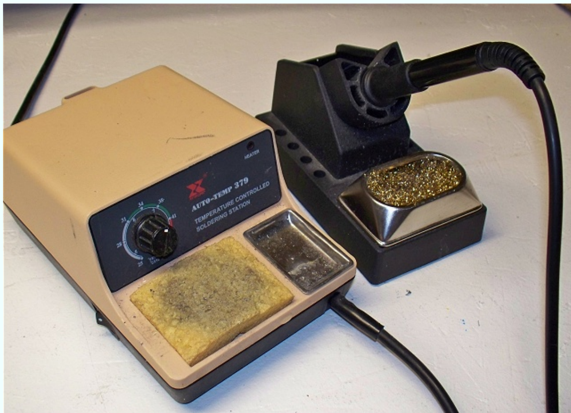
Figure 2-10. Typical temperature-controlled soldering station
