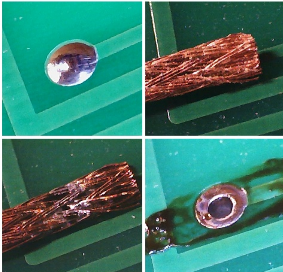
Figure 2-17. Clearing a pad's hole with desoldering braid
