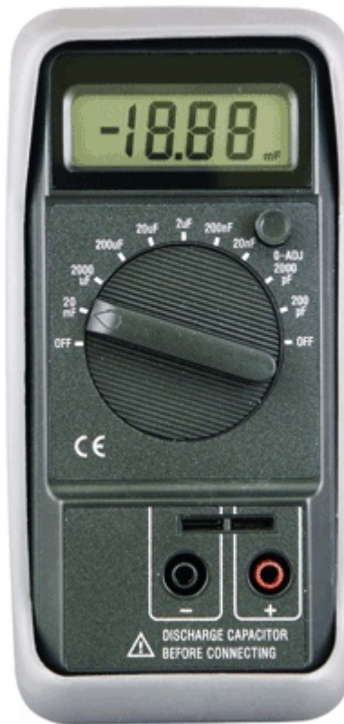
Figure 2-7. A typical capacitance meter
