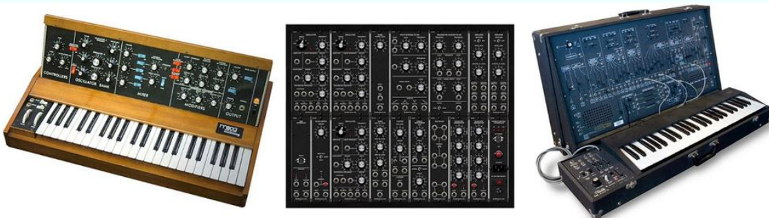
Figure 3-1. Analog synthesizer modules vary in size, but are generally about two to four inches wide by eight or so inches tall. The faceplates bristle with cryptic legends, knobs, switches, buttons, and LEDs. Each one performs a particular function and has clearly marked inputs, outputs, and controls. The Mini-Moog (left) is an example of a normalized synth. The Synthesizers.com synthesizer (center) is a modular synth, and the ARP 2600 (right) is a hybrid of the two types.
